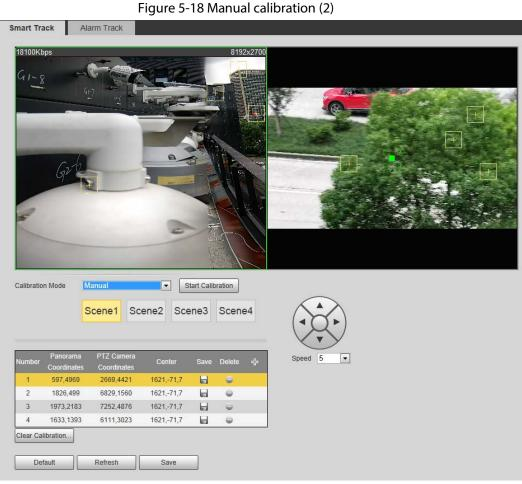
1) Adjust the speed dome lens and turn it to the same view as the chosen lens, and then click 🖶.
