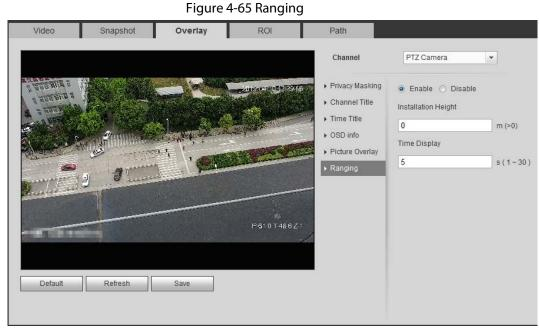
Step 2Select the **Enable** checkbox, and then set the installation height and time display.Time display: The display time of the ranging information on live image.
